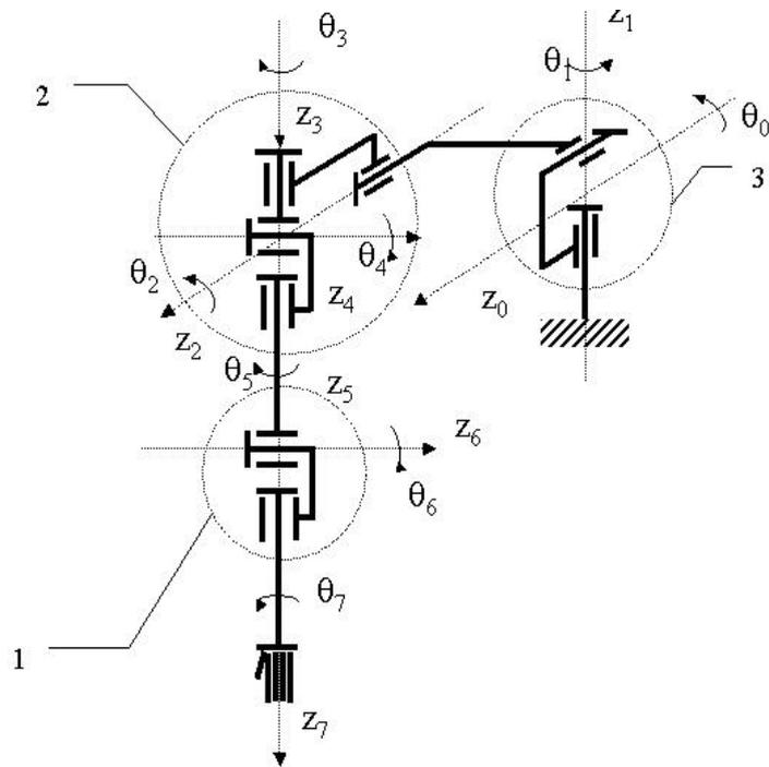
To a bigger part it is dependant to the requirement the dummy limb to be as close as possible to the shape and parameters of the human arm. There is a potentiometric sensor built in each kinematics couple for measurement of the current joint coordinate. The imitation of muscle resistance (spasm) is executed by DC motor-gearboxes and servo brakes. The change of the forces and torques of the fore and upper arm joints is measured by 6 component F/T sensors.
