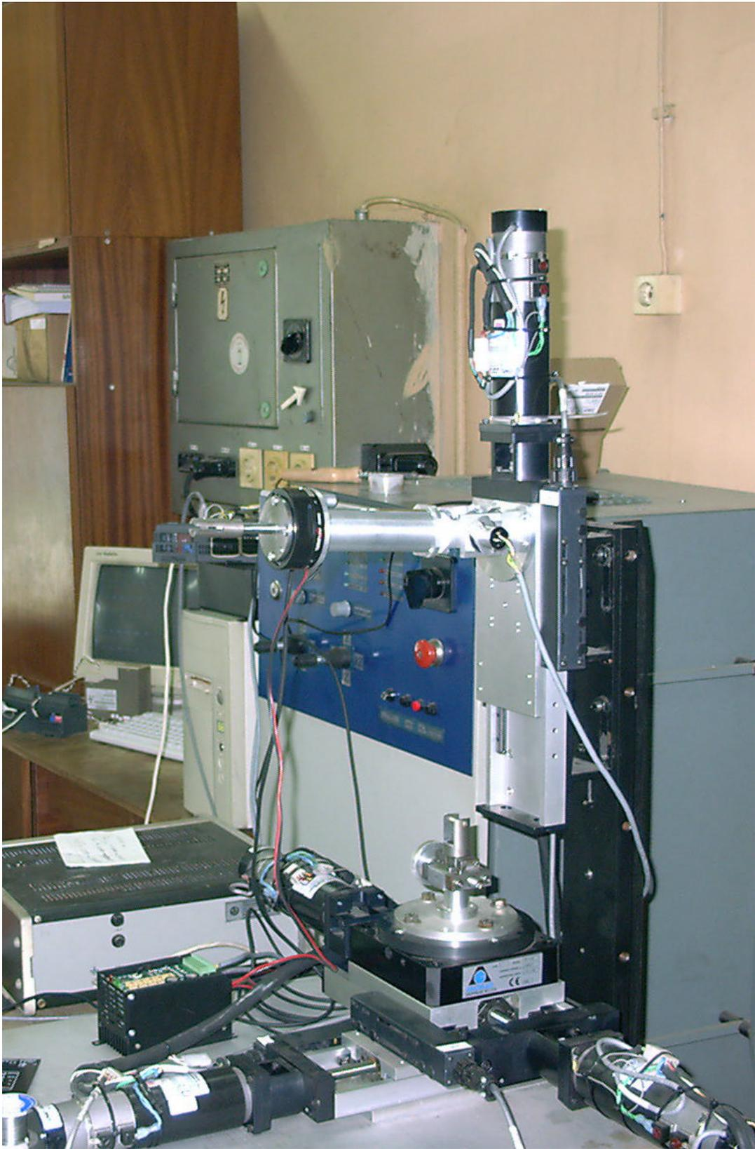
Photo 11 – The forearm attached to the test-bed
