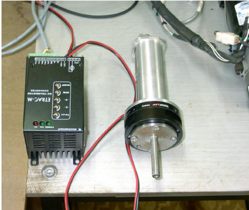
Photo 9 – The base of the assembled forearm with the DC motor controller
